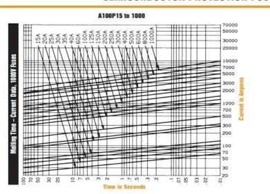
Example: 800V system requires a 1000V "A100"-style fuse, if it is a 10 second application of battery power at 1000amps, you require approximately a 300Amp battery fuse.
