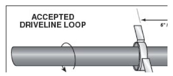
DRIVESHAFT TUBE DEFINITION: Driveshaft must be covered by a 360-degree round, oval, or tapered tube, covering the front U-joint and extending rearward a minimum 12 inches. Minimum thickness of tube is .050-inch steel or titanium. Driveshaft tube must utilize a minimum of four attachment points to the chassis, using either minimum 5/16 SAE Grade 8 bolts, welded, or 1/4-inch push/pull pins. Two-piece tube assembly permitted with a minimum of six 3/8-inch SAE Grade 8 bolts.
